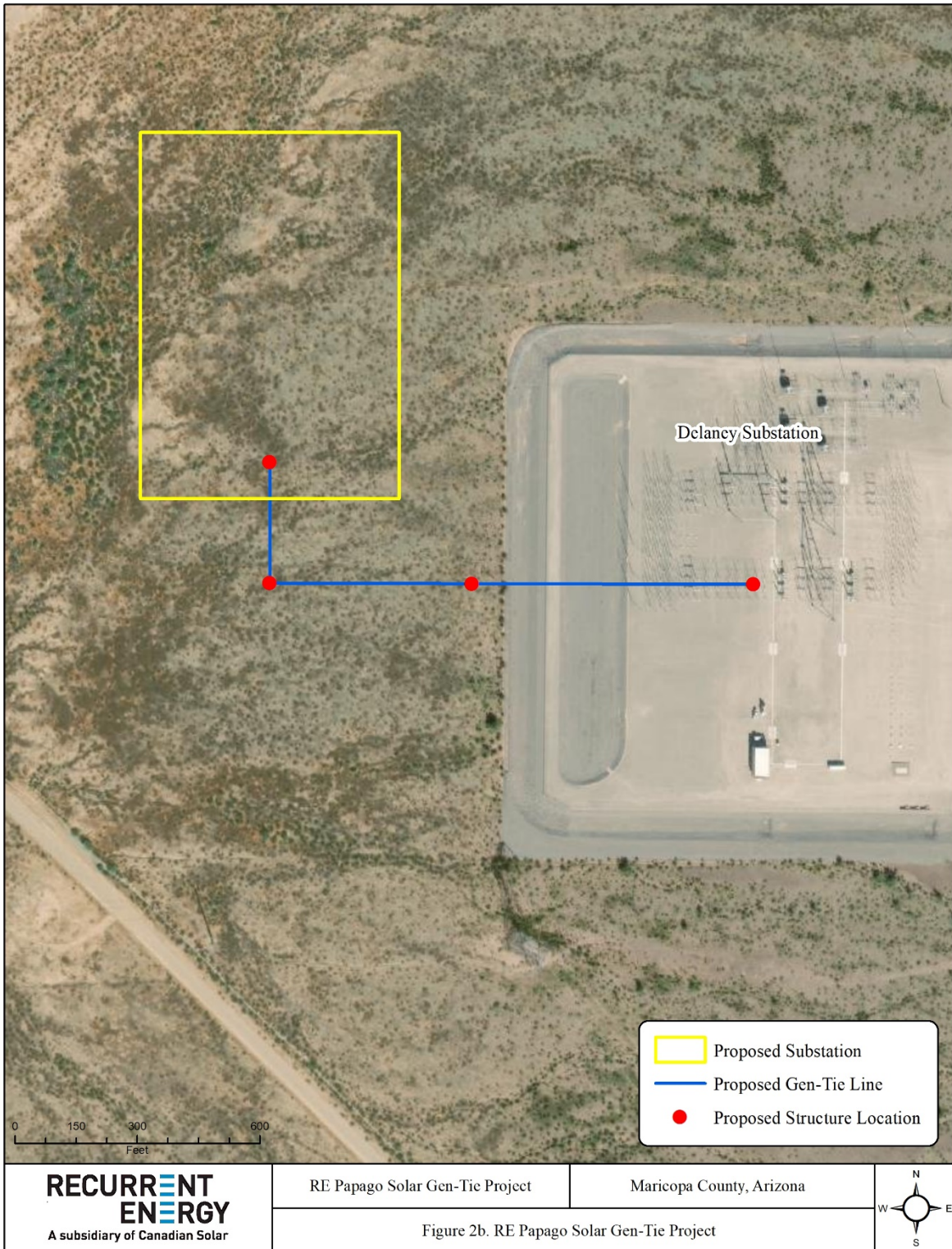
Figure 2b. Alternate conceptual project substation and gen-tie line location map showing a potential offset connection to Delaney Substation requiring the utilization of a turning structure
