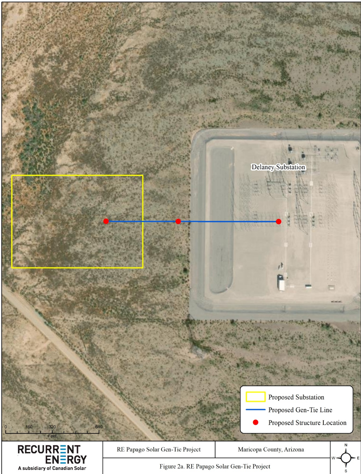
Figure 2a. Conceptual substation and gen-tie line location map showing a linear connection to Delaney Substation
